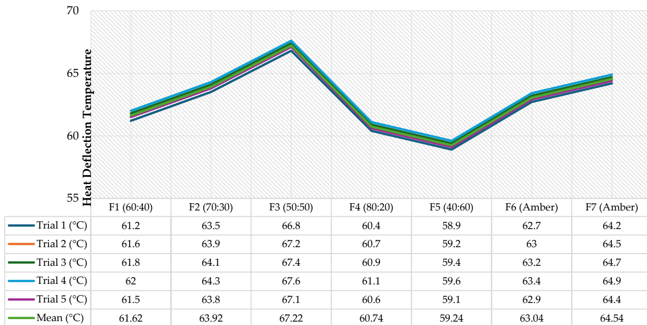
Figure no. 7: Evaluation of blends by Heat Deflection Temperature (HDT)
